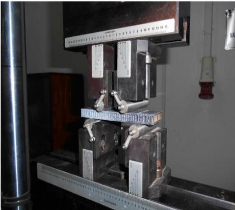
**Figure 7** – Four Point Bending Test carried on honey comb specimen (max load)
