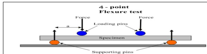
**Figure 5** – Schematic showing individual forces in a 4 Point Flexure Test
