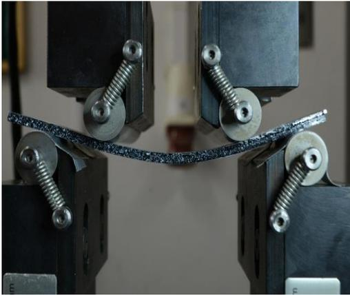
**Figure 6** – Four Point Bending Test carried on honey comb specimen (Zero Load)
