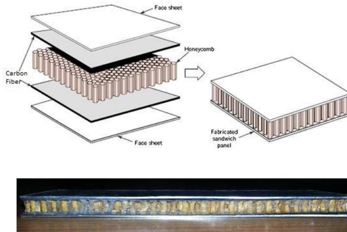
**Figure 4:** Assembling elements
