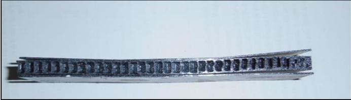
**Figure 12:** Honeycomb Structure (Delaminated)
