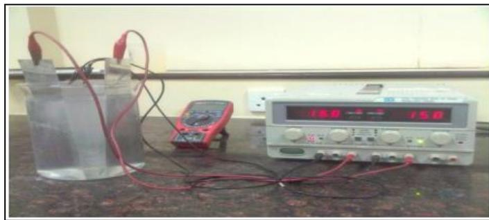
**Figure 3:** Surface treatment process for adonization of Aluminum
