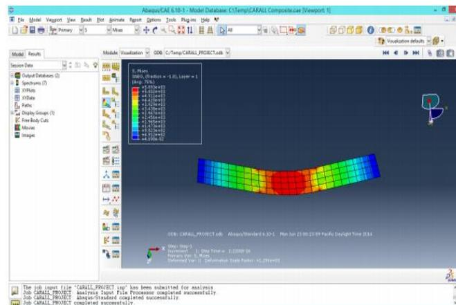
**Figure 14:** Simulation result of CARALL
