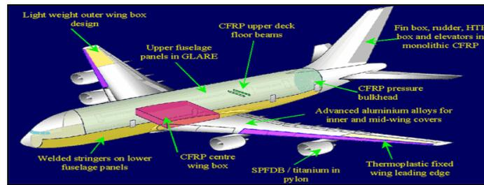
**Figure 2:** Upper fuselage shell of the A380 airplane using GLARE as the main composite
