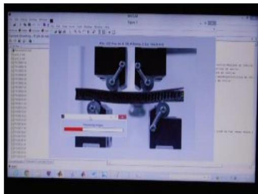
**Figure 11:** Digital Image Correlation Process in MATLAB
