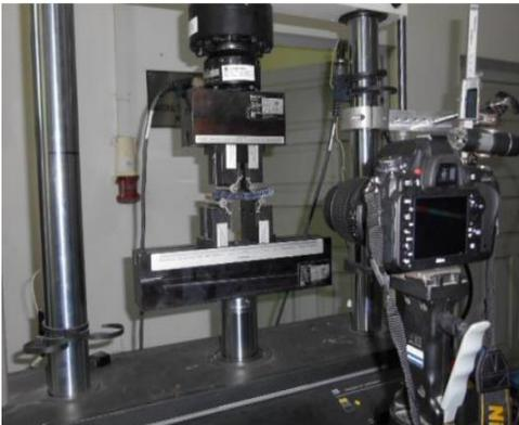
**Figure 9** – Four Point Bending Test carried on CARALL specimen (max load)
