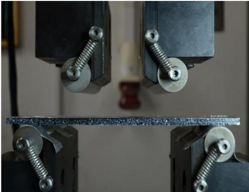
**Figure 8** – Four Point Bending Test carried on CARALL specimen (Zero Load)
