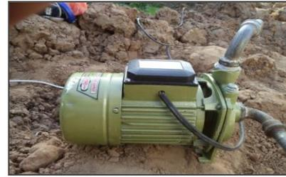
Figure 3: Electric circular pump
